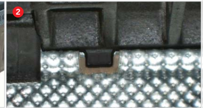
Align anti-shunt detail with recess
