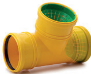
KDR 27 triple drainage junction with \varnothing 110 connector connects \varnothing 72 - \varnothing 100 mm drainage pipes
