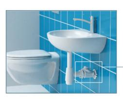
The non-return valve in version B is connected to the  $\emptyset$  50 pipe socket of an existing pipe fitting in the wall. A special aesthetic masking rosette allows the valve to be mounted to the wall by means of two screws. This protects the system from self-detachment in cases of increased pressure in the system caused by sewage backflow. To the device mounted in such way, the trap (e.g. a washbasin) is to be connected by means of a special connector with a screw cap.
