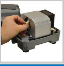
Gently remove one of the magnet bar ends by pulling it out of the housing, being careful not to scratch or break the housing or magnet bar.
