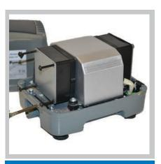
Put chamber cover back and screw four screws in. Repeat with other chamber cover.
