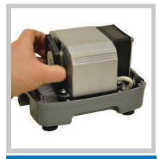
Remove the screw along with the diaphragm depressor, electrostatic membrane and diaphragm. Repeat on the opposite end of the pump.
