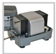
Unscrew the four corner screws from the chamber cover at one end of the pump. Seperate the chamber cover at the seam to expose the screw holding the white round plastic diaphragm depressor in place.
