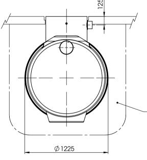
225mm (Min.) Concrete surround around tank body for units up to 1.0m inlet invert.
