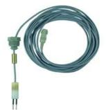
The supplied conductivity Level Probe is used as a minimum water level detector in the rainwater tank. The standard length of cable supplied is 15m. This can be extended to order, up to 100m. It carries a very low voltage/current.
