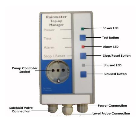
**Test button:** Pressing this when the Solenoid Valve is closed will momentarily open and close the Solenoid Valve.
