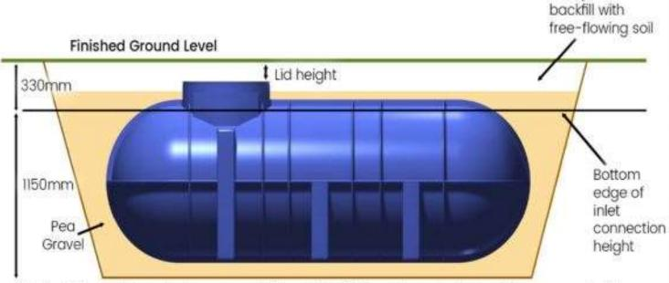
Bed on 50mm of rounded pea-gravel & backfill to 50mm above tank top with same material
