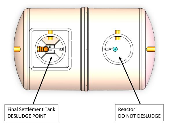
Insert the suction hose into the FST, taking care not to damage the sludge return pipework. Approximately 300mm of active sludge must remain in the bottom of the reactor.
