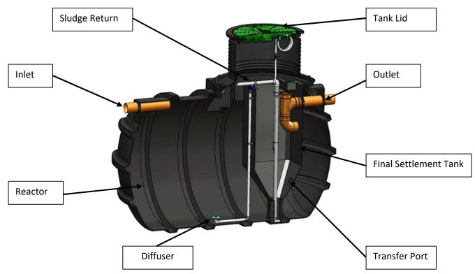
The main casing and cover of the BioAir are constructed of Medium Density Polyethylene.
